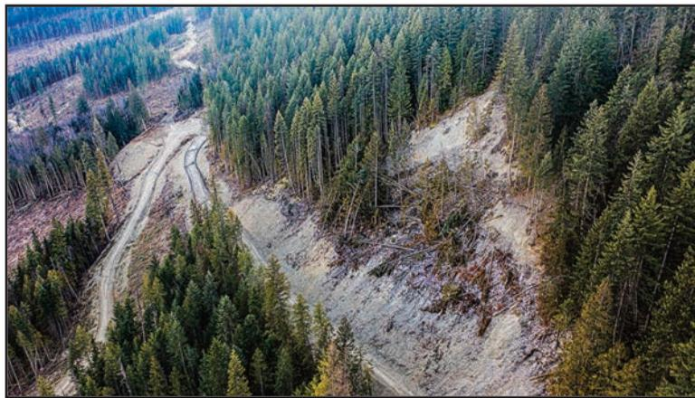
**One of three landslides caused by clearcutting and the construction of a \$4.8 logging road on steep slopes above Duncan lake. Continued road construction means more logging is in store for the park proposal. [Photo: Isaac Carter]**
